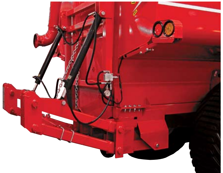
LEVEL-LIFT System and manure pipe quick coupler
