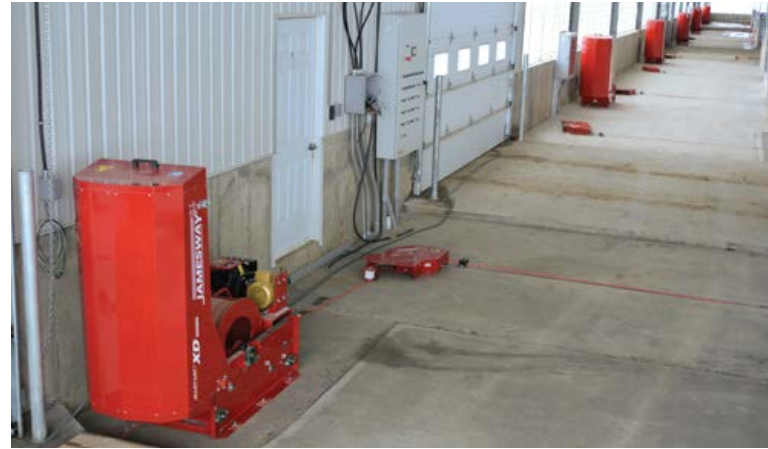
The Jamesway Scraper-Boss PRO can operate up to 4 alley scrapers.
