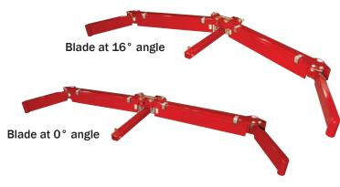
When operated at 0° angle (fully straight), Jamesway Straight blades will require the least amount of space at the ends of the barn. The same blade may also be set to operate at 16° angle to keep the manure load centered when used in drier conditions.
