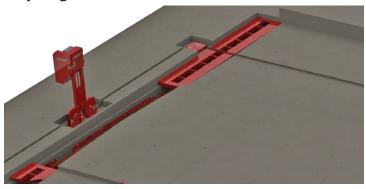
Modular Gutter Covers are used to cover the manure gutter in the scrape alleys. These 12" or 18" wide heavy duty modules are laid across the gutter width, allowing easy removal of individual segments. The 9" opening allows manure to fall through yet tractors or skidsteer loaders can easily drive over.
