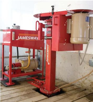
The Electric Prop Agitator is ideal for preconditioning bedded manure when transferring to storage with the Jamesway Liqui-Trans piston pump. Likewise, centrifugal transfer pumps will experience fewer problems with blocked inlets, and gravity-flow systems perform better with homogenous material. The uniform consistency of manure blended with the Jamesway Electric Prop Agitator also helps keep separator systems operating at peak efficiency.
