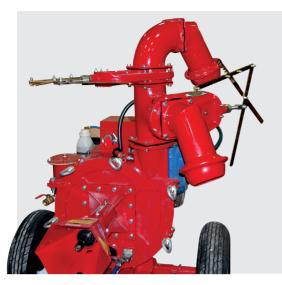
Jamesway offers a wide range of 6" and 8" accessories to complete your Vacu-Pump connections. Outlet accessories can be assembled in endless combinations to fit every need. These heavy duty components are rock solid and powder-coated for long life. The inlet vacuum hose is equipped with a camlock quick connector for easy set up. Choose either the strainer inlet for pits or choose the quick coupler for truck transfer connections.
