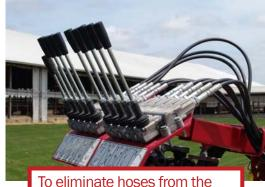
control stand, cable-operated spool valves are a good choice when there are many functions.
