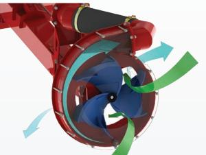
The center of the PUMPELLER turbine is a propeller that creates a powerful intake suction that pulls in tough solids and obliterates them at up to 50 cuts per second. The integral impeller blades on the outer edge deliver fast load-out and high cannon pressure.
