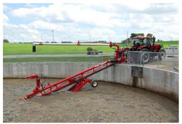
Heavy pumps need heavy undercarriages so every wheel kit sits on an  $8"\ (20\ cm)$  pivot and has dual lift cylinders.
