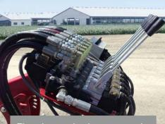
Electric spool valve operated from control box inside tractor. Use with wired or wireless controls.
